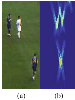
Fig. 3 Example of parallax errors. (a) Crop of a camera view with 3 targets. (b) Corresponding detection volume showing 3 high intensity regions (the targets) and a 4 th region generated by parallax error.
