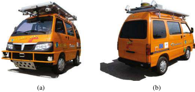
Fig. 2 Front and back views of the electric vans used during VIAC, with accessible sensors.
